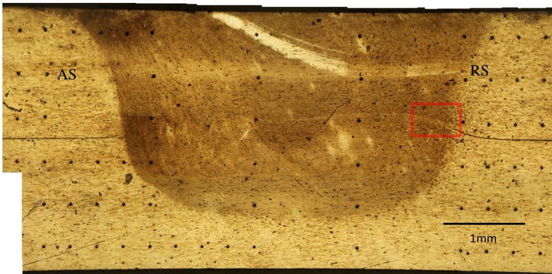
Figure 3.31 Metallographic picture of SSFSW #3763 welding sheet cross section at -1500 rpm, 8.47 mm/sec, 9.79 kN tool 2(RH)
