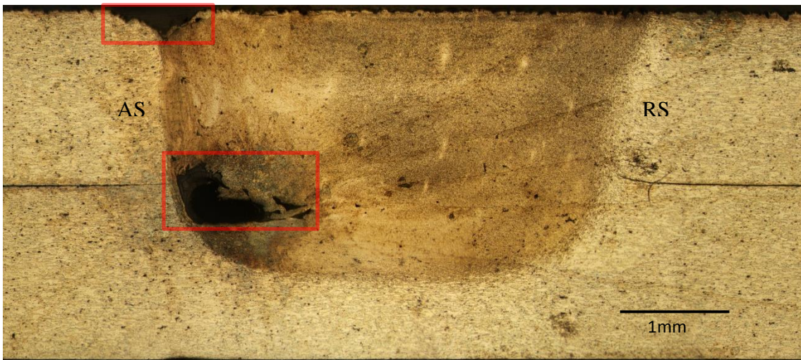
Figure 3.29 Metallographic picture of SSFSW #3760C welding sheet cross section at -1800 rpm, 8.47 mm/sec, 9.79 kN tool 1(RH)
