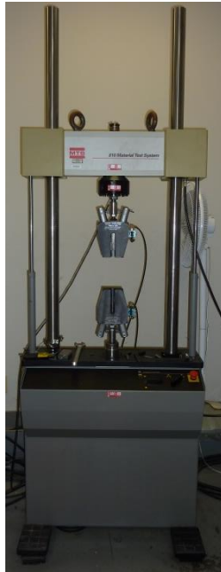
Figure 2.23 MTS 810 tensile test machine
