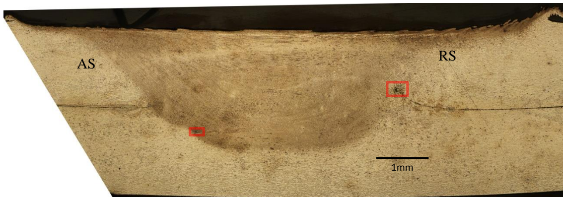
Figure 3.34 Metallographic picture of CFSW #3884 welding sheet cross section at -1500 rpm, 8.47 mm/sec, 6.67 kN tool 4(RH)
